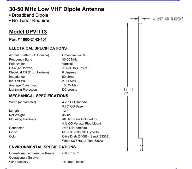
The DPV-113 is a 30-50 MHz broadband, passive, vertically polarized dipole that does not require a tuner for operation. The antenna is designed to withstand and operate in a worse case wind loading of 150 MPH wind with no ice.
